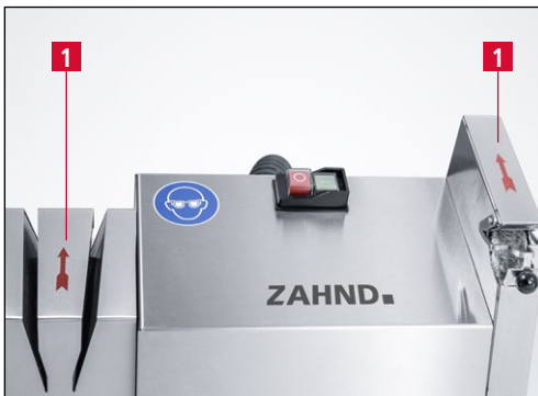
Figure 6-2 Checking rotating direction
