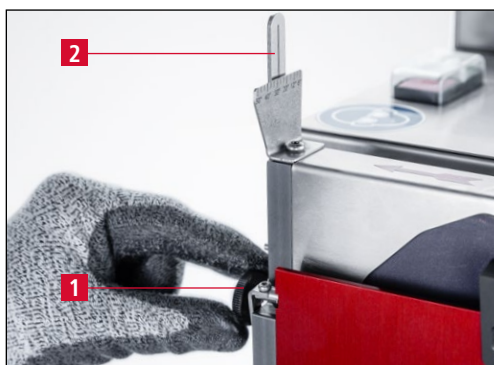
Figure 7-2 Setting the grinding angle
