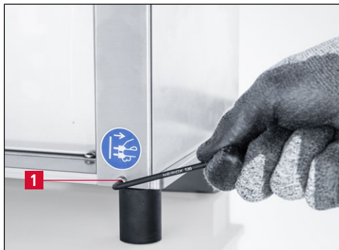
Figure 7-14 Loosening the polishing disk cover at the front
