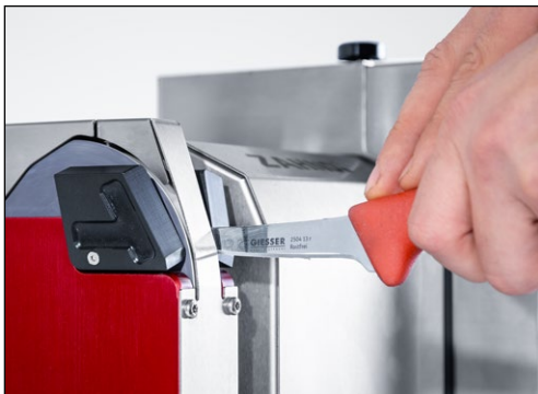
Figure 7-4 Sharpening hand knives
