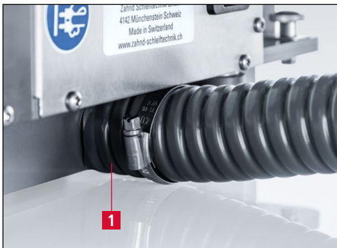
Figure 3-4 Dirt tray with suction nozzle
