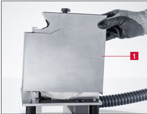
Figure 7-15 Removing the polishing disk cover
