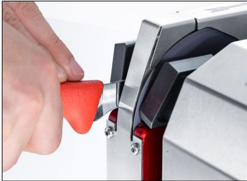
Figure 7-3 Sharpening hand knives
