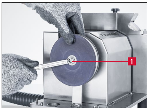
Figure 7-10 Loosening the screw
