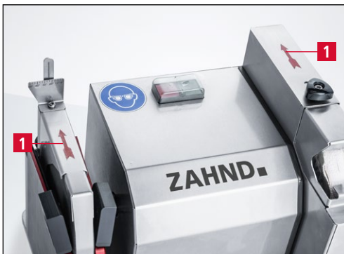
Figure 6-2 Checking rotating direction
