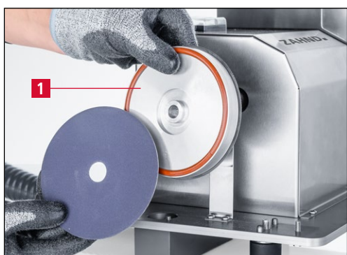
Figure 7-12 Mounting a new pair of grinding wheels
