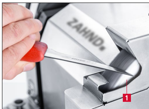
Figure 7-6 Deburring and polishing hand knives
