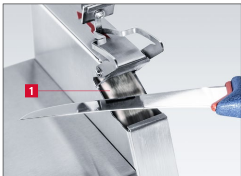
Figure 7-6 Polishing hand knives
