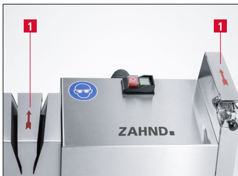
Figure 6-2 Checking rotating direction
