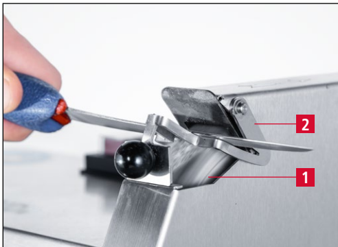
Figure 7-9 Polishing hand knives
