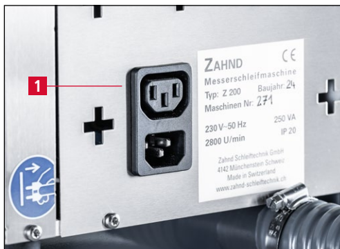
Figure 7-23 Connection for industrial vacuum cleaner
