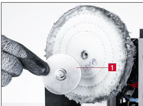
Figure 7-19 Removing the clamping screw and clamping flange
