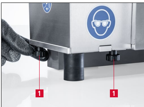
Figure 7-10 Unscrewing the knurled nuts
