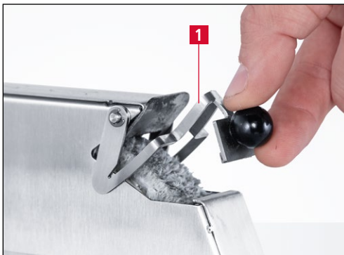
Figure 7-4 Folding the guide bracket upward
