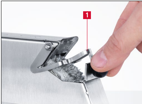
Figure 7-8 Folding down the guide bracket
