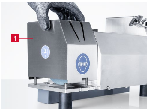
Figure 7-11 Removing the protection hood
